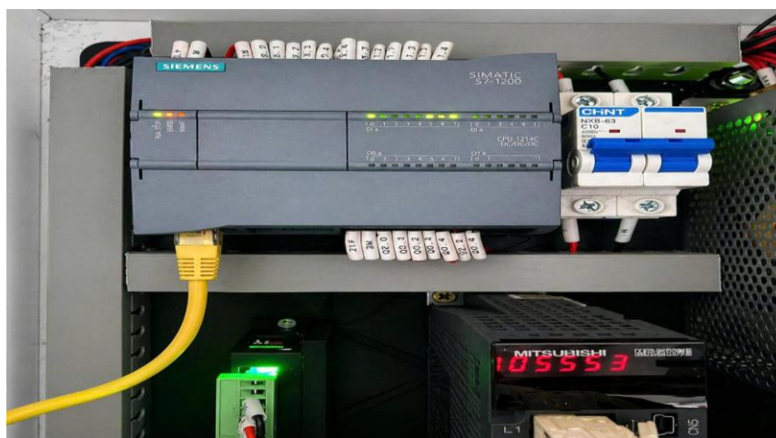
Fig. 2. PLC–servo driver wiring for Siemens S7-1200 and Mitsubishi servo system.
