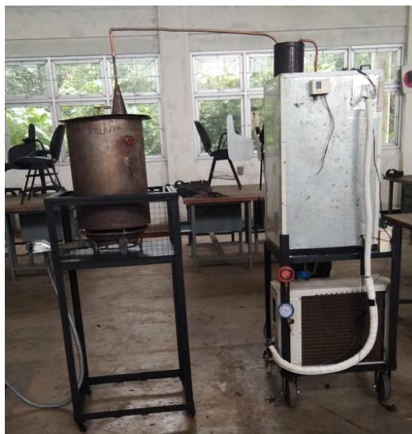
Fig. 1. Smoke condensation using a low temperature air media refrigeration system
