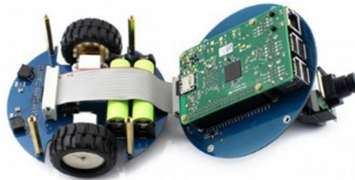
Fig. 6. Raspberry Pi is mounted on the AlphaBot2 chassis using standoffs and connected via GPIO.
