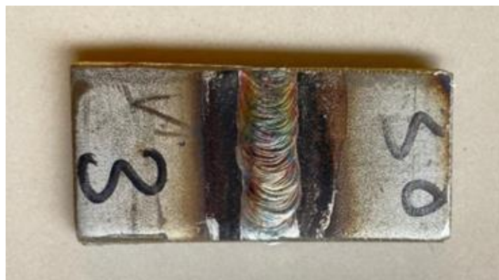
Fig. 3. Shape of Test Specimen after the welding process.
