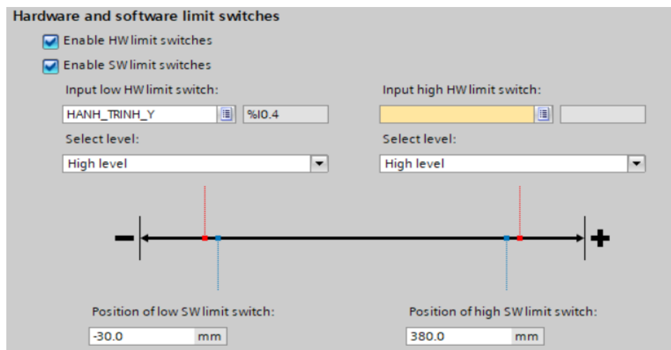
Fig. 13. Setting the Y travel limit
